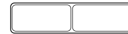
65 x 16 x 1.2mm SLAT with Centre Support Gusset (Lengths 1800mm; 2400mm; 3600mm)
